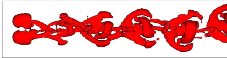
Fig. 10. Vortical structure at Re = 300 for h = 1.5D [29].
